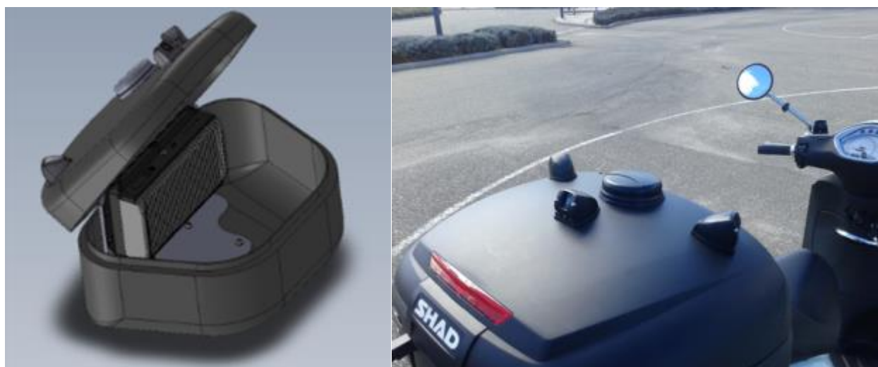
Figure 19 and Figure 20: Topcase for PTWs, showing the DAS, 3 cameras and GPS antenna
