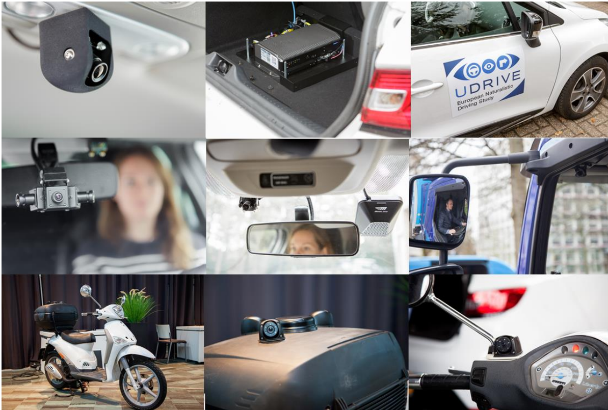
Figure 3.2: Illustration of UDRIVE DAS and the integration in different vehicle types.
