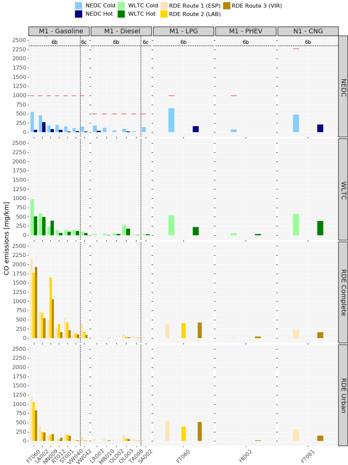
Figure 5: CO emissions for Euro 6b and Euro 6c vehicles over the NEDC laboratory cold and hot tests (top panel), the WLTC laboratory cold and hot tests (second panel) and on-road tests (third panel for complete trip and bottom panel for urban section). On the top panel, horizontal red lines stand for the CO limit applicable on the Cold NEDC.
