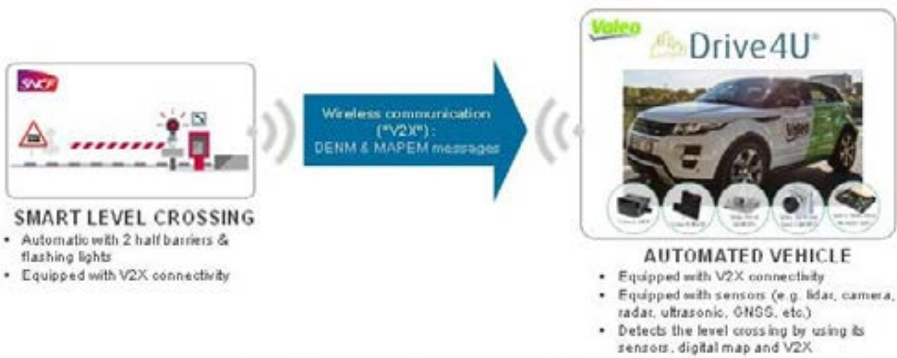
Preparing level crossings for the arrival of automated vehicles (Virginie Taillandier et al. in TS8: Traffic Management Safety)
